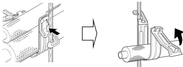
NOTE: When removing SRV from W3/8" threaded rod, open the lid, then remove it.
