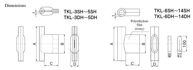
• Material: Polyethylene foam with factor of 30
