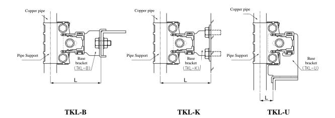
Distance L between the center of copper piping riser and the base bracket (wall) (inch)
