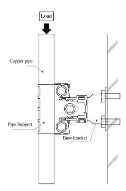
Note: The load capacity indicates the load that the test piece is capable of supporting the copper pipe when load is given to that test piece.
