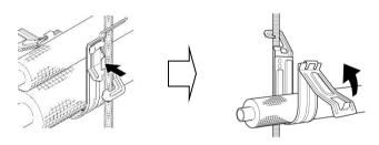
NOTE: When removing SRV from W3/8" threaded rod, open the lid, then remove it.
